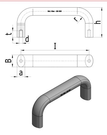
$\begin{array}{lll} a & = 17 \\ b & = 26 \\ d & = M8 \\ h & = 55 \\ I & = 117 \\ r & = 17 \\ t & = 12 \\ Weight in (g) = 170 \\ \end{array}$
